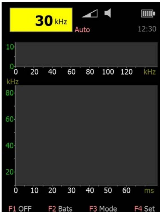
Menus und submenu are reached by pressing the buttons F1 to F4:
